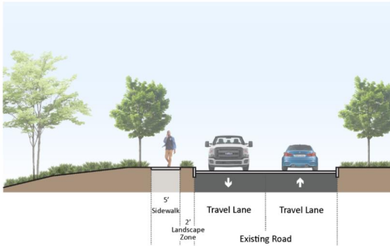
Figure 16.6.B.2.a – Sidewalk Cross Section 1
