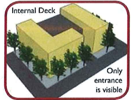
Wrapping the deck with development hides it from view
